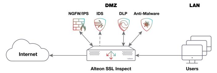
Figure 1: SSL Inspect steers traffic to active inline security inspection tools (NGFW, IPS, DLP) as well as to passive, out-of-path, security inspection tools (IDS)
